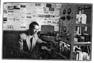
CTIBW scored 89,262 points for an All-Band total. You should remember Leonel as CR5UP. His rig was running about 50 watts input at that time but is now capable of 150 watts or so. Two receivers were used, an 11 tube Eddystone 5750, and a 13 tube home built job with dual conversion. Antenna is for multi-band work on 7, 14 and 28 mc, and is fed with a 600 ohm
