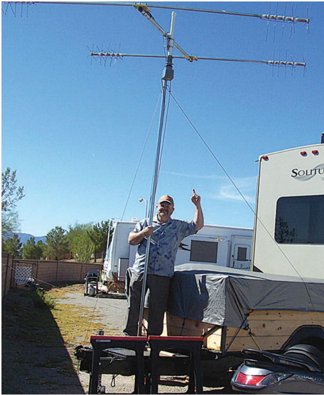
Eddie, AE7AE, worked several hundred QSOs on 10 meters using this mini-beam that is only 12-feet high. (Courtesy of AE7AE)
