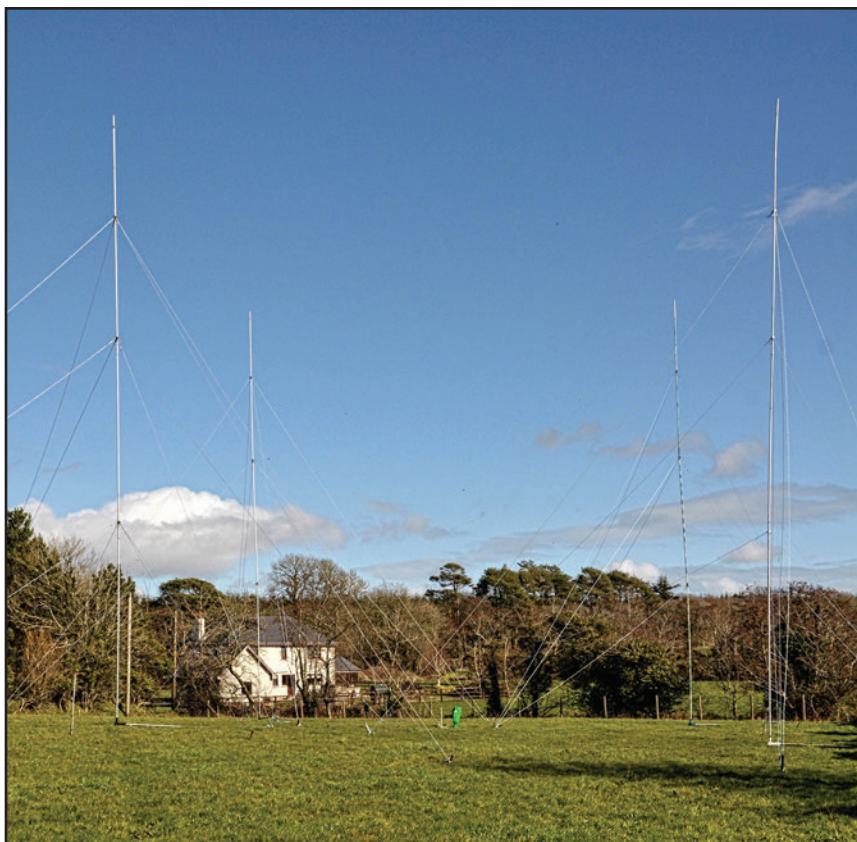
The 80-meter 4-square antenna used by EI5DI for his single-band effort. (Courtesy of EI5DI)
